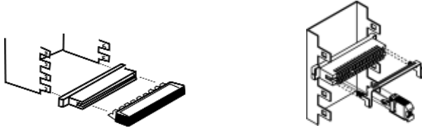
ONEAC OnLine 10-Series (10 line and 1 line) protectors are designed to fit easily into Krone LSA-PLUS™ connection strips on the frame.
